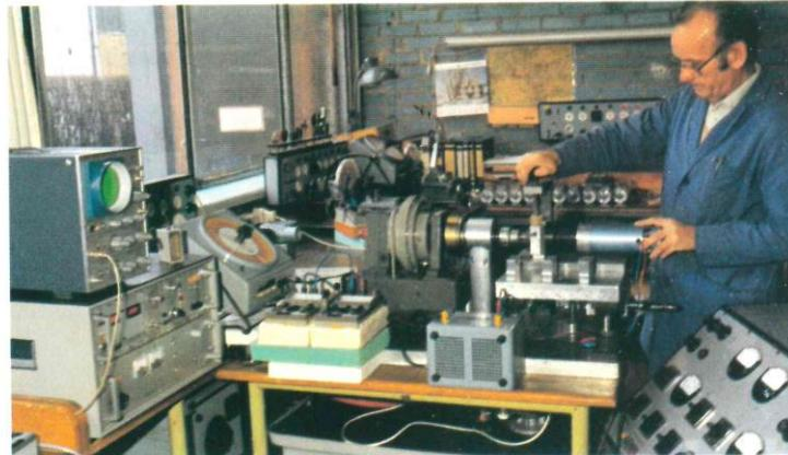
production stages, followed finally by the final inspection procedure after final assembly on production testing rigs. These procedures are accompanied by fatigue tests using special measuring rigs and gauging machines.
